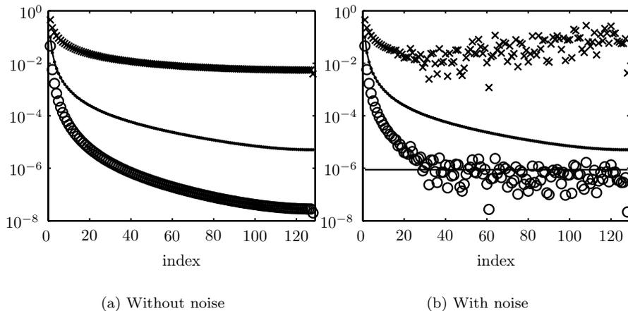
Figure 2.2: The dots show the singular values of an  $128 \times 128$  DERIV2 problem. The circles (o) show the coefficients  $|\mathbf{u}_i^T \mathbf{y}|$ , while crosses (x) show solution coefficients  $|\mathbf{u}_i^T \mathbf{y} / \sigma_i|$ . The noise dominates the small coefficients and the corresponding solution coefficients are too large because of small corresponding singular values. The straight line in (b) shows  $\delta$ .
