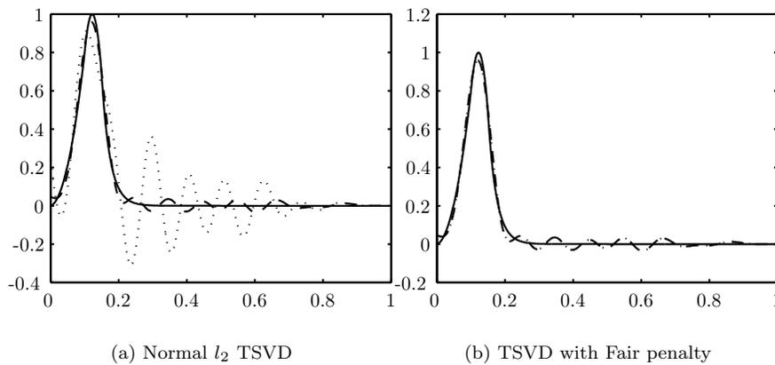
Figure 3.7: Standard and robust TSVD with truncation parameter  $k = 20$  applied to problems with outliers (dotted solution) and without outliers (dashed solution). The test problem is described in Fig. 3.6 and is also solved via variations of Tikhonov in Figs. 3.9 and 3.10.
