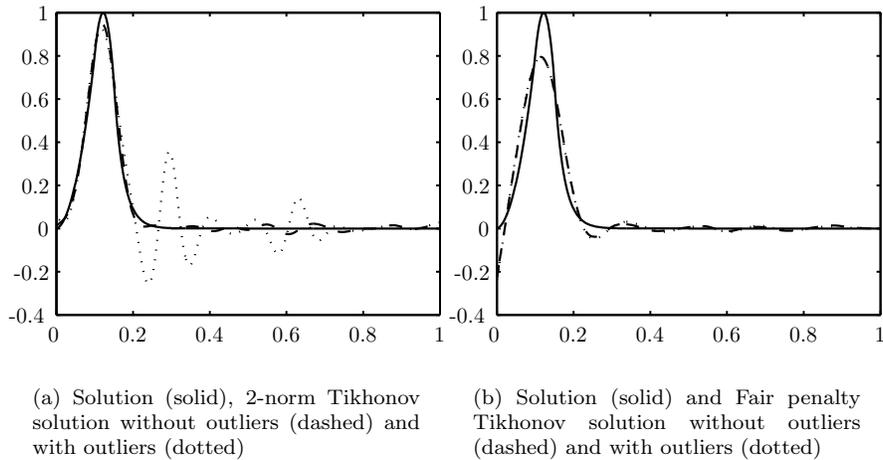
Figure 3.9: Robust Tikhonov regularization solutions. The test example is HEAT,  $\mathbf{K} \in \mathbb{R}^{300 \times 300}$ . White noise  $\|\mathbf{e}\|_2 = 10^{-2}\|\mathbf{y}\|$  and three outliers are added to the right-hand side, see Fig. 3.6. The regularization matrix is  $\mathbf{L}_2$  and the regularization parameter is  $\lambda = 10^{-1}$  in both cases and has not been optimized.
