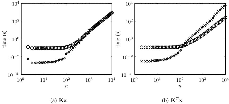
Figure 4.4: Timings of object oriented penalty. Timings for 300 multiplications  $\mathbf{K}^T \mathbf{x}$ , where  $\mathbf{K} \in \mathbb{R}^{n \times n}$  with object oriented techniques (o) and without ( $\times$ ). The computations were performed in Matlab 6.1.
