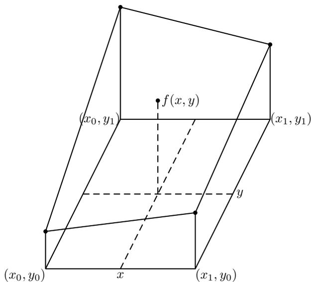
Figure D.2: Geometry of interpolation
