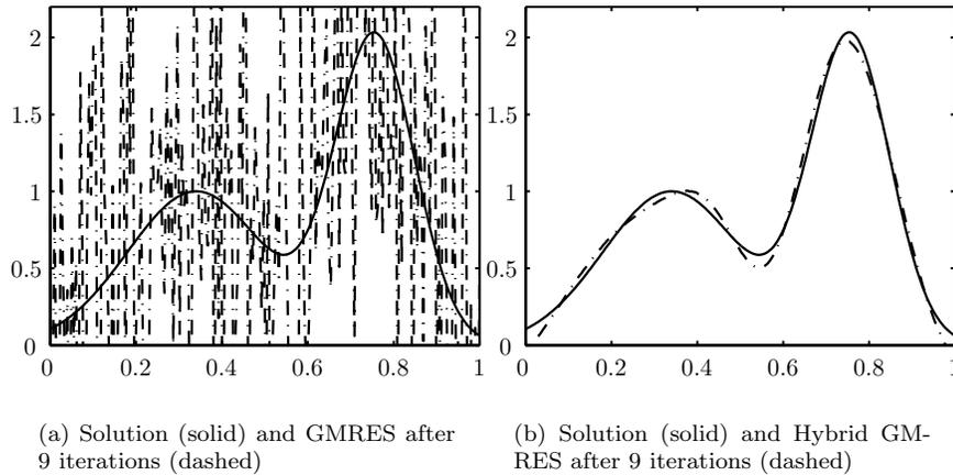
Figure 3.5: The GMRES and hybrid GMRES-Tikhonov methods on the SHAW test problem with  $\mathbf{K} \in \mathbb{R}^{200 \times 200}$ . Normal distributed noise with norm  $10^{-3} \|\mathbf{y}\|_2$  is added to the right-hand side. The GMRES solution explodes in the 9th iteration (one to many). The hybrid method uses Tikhonov regularization with the GCV parameter choice method.
