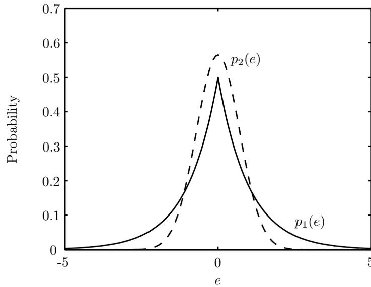
Figure 2.4: The normal probability density function  $p_2(e) = \exp(-e^2)/\sqrt{2}$  (dashed line) and the  $l_1$ -norm probability density function  $p_1(e) = \exp(-|e|)/2$  (solid line). The normal density function is more concentrated around 0 than the Laplace distribution function that instead has larger and longer tails.
