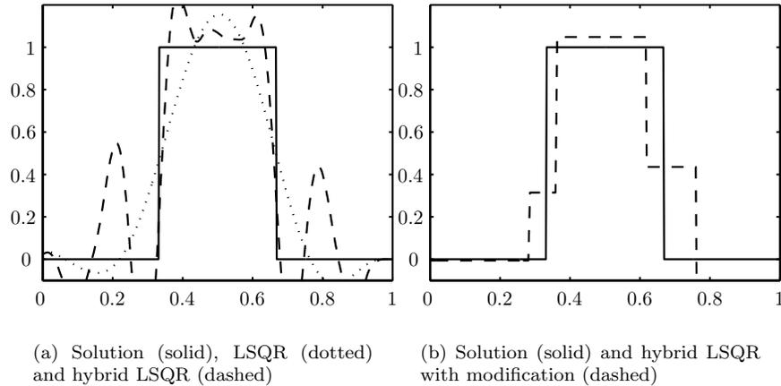
Figure 3.8: LSQR, hybrid LSQR and hybrid LSQR with modification—all after 7 iterations. The example uses the HEAT problem with  $\mathbf{K} \in \mathbb{R}^{400 \times 400}$ , a piecewise constant solution and normal distributed noise with norm  $10^{-2} \|\mathbf{y}\|_2$  is added to the right hand side.
